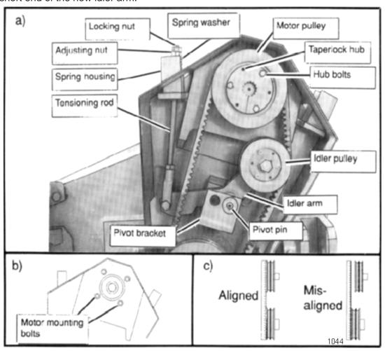
Reinstall the idler arm and pivot pin. The pivot pin is installed into the hole in the pivot bracket closest to the idler pulley. When assembling for **standard** cut rotation, the idler arm is installed with the idler pulley toward the front of the mower with the pivot pin in the front hole. When assembling for **reverse** rotation, with smooth cut knives, the idler arm is installed with the idler pulley toward the rear of the mower with the pivot pin in the rear hole.
